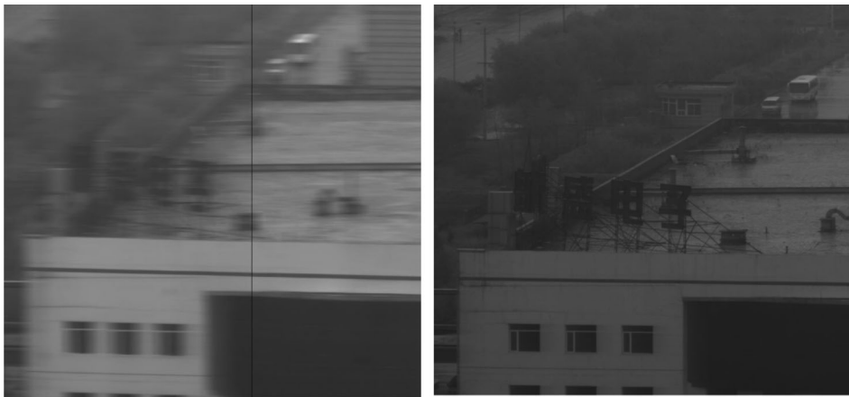
Figure 10. Comparison of image motion compensation experimental photographs: (a) without image motion compensation and (b) with image motion compensation.
