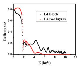
Fig. 5. Reflectance curve of the supermirror with an energy step of 1.0 keV at 1.4 degree.
