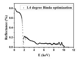
Fig. 8. Reflectance curve of the supermirror further optimized by Binda genetic algorithm at 1.4 degree.
