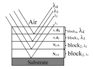
Fig. 1. The sketch for the principle of block method.
