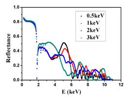
Fig. 4. Reflectance curves of supermirrors with energy steps of 0.5, 1.0, 2, 3 keV at 1.0 degree.
