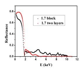
Fig. 6. Reflectance curve of supermirror with an energy step of 1.0 keV in 4–7 keV and 0.5 keV in 8–10 keV at 1.7 degree.
