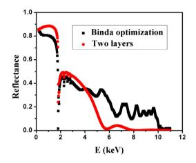
Fig. 7. Reflectance curve of the supermirror further optimized by Binda genetic algorithm at 1.0 degree.
