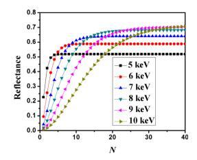
Fig. 2. Reflectance curves as a function of the number of layer pairs in 5-10 keV at 1.0 degree.
