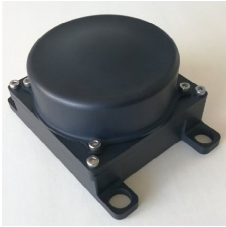
Fig. 9. Flywheel integrally designed with isolator.
