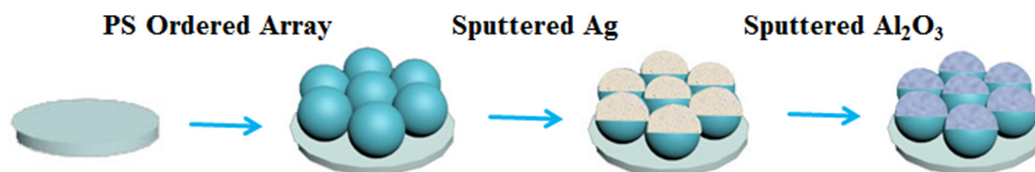
Fig. 1. The schematic of the fabrication process for PS/Ag/Al 2 O 3 ordered arrays.
