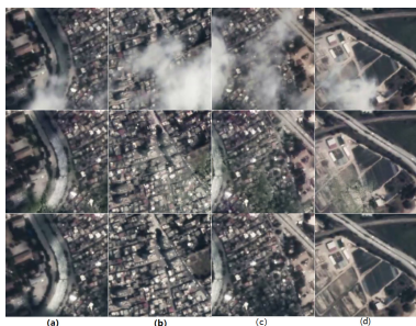
Fig. 3. Removal result of CAGN on real cloud images. (a)–(d) We select four images to illustrate. Each row from top to bottom corresponds to the cloud image, the result of CAGN, and ground truth.
