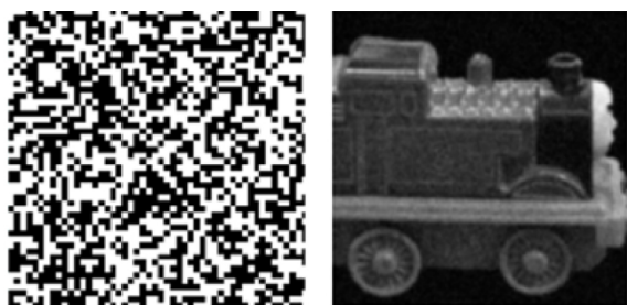
(a) CASSI 系统恢复图和编码模板 (a) Recovery diagram and coding template of CASSI system
