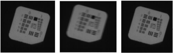
图 14 平台扫描速度为 5(°)/s 时,几种情况的像移补偿效果对比 Fig. 14 Comparison of image shift compensation effect for three different conditons with platform scanning speed of 5(°)/s
