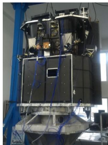
Figure 6. The lift-off vibration test of the satellite.
