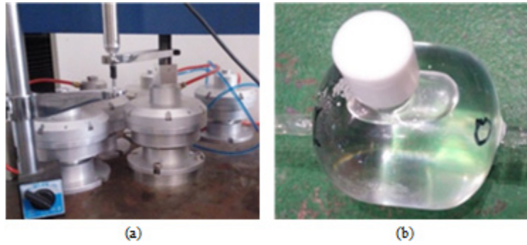
Fig. 4. Testing a 5-unit group: (a) group with 5 HSUs in test; (b) vapor buffer bottle.
