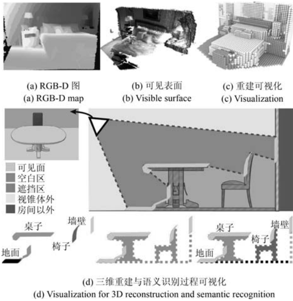
图 1 本文深度卷积神经网络的场景重建与语义分类过程 Fig.1 3D reconstruction and semantic classification of our depth convolutional neural network
