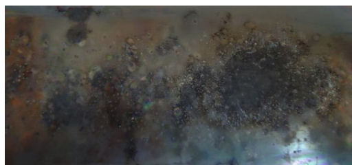
Fig. 7. discharge electrode after ablation by arc discharge.
