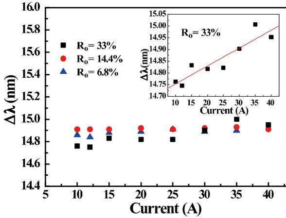
Fig. 8. The spectral width  $\Delta\lambda$  as a function of current for the SBC of laser array with different OC reflectivity. The inset is the zoom-in curve for SBC with OC reflectivity of 33%.
