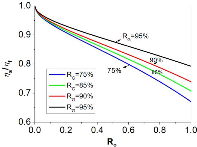
Fig. 4. The influence of diffraction efficiency of grating  $R_G$  on the ratio of  $\eta_s/\eta_t$  with different OC reflectivity  $R_o$ .
