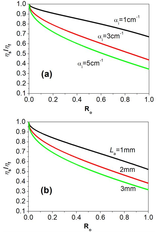
Fig. 3. The ratio between energy conservation efficiency of SBC and free running ( $\eta_s/\eta_f$ ) as a function of  $R_o$  with different (a) internal loss  $\alpha_i$  and (b) cavity length  $L_a$ .
