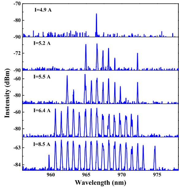
Fig. 6. Lasing spectra of SBC with OC reflectivity of 14.4% at different current.
