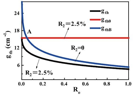
Fig. 2. Threshold modal gain as a function of the OC reflectivity.
