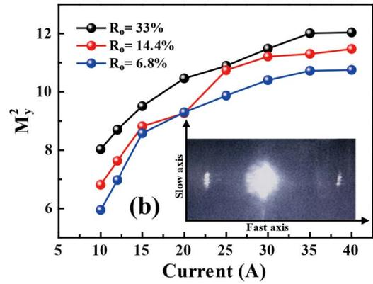
Fig. 10.  $M^2$  factor in (a) the fast and (b) slow axes of SBC laser with OC reflectivity of 33%, 14.4% and 6.8%. The inset in (b) shows the far-field pattern of SBC with OC reflectivity of 6.8%.
