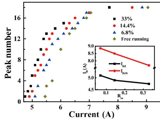
Fig. 7. Lasing of single emitter in free running and SBC with OC reflectivity of 33%, 14.4% and 6.8% as a function of injected current. Inset shows the dependence of threshold current of single emitter on the OC reflectivity  $R_o$ .
