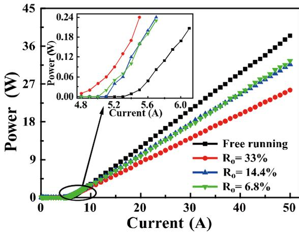
Fig. 5. Power performance of laser array under free running and SBC with different OC reflectivity. The inset shows the threshold characteristics.
