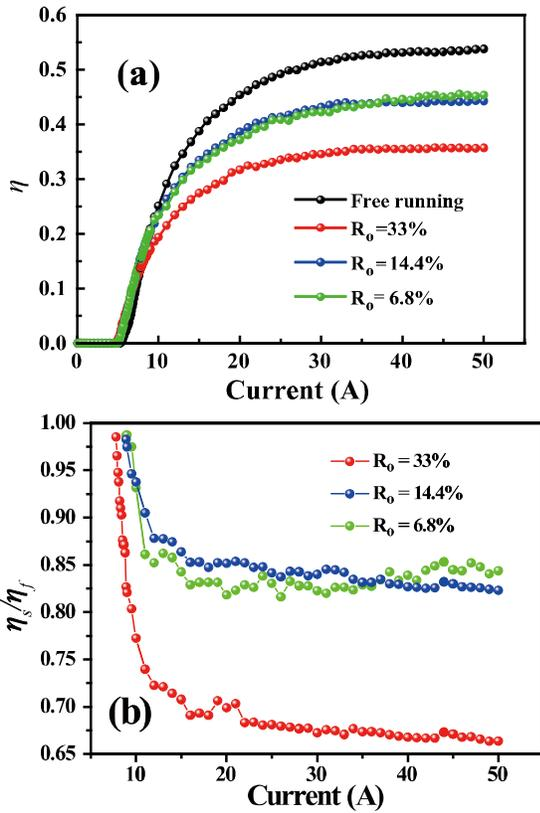
Fig. 9. (a) Energy conversion efficiency  $\eta$  and (b) combining efficiency  $\eta_s/\eta_f$  of laser array under the free running and SBC operation with  $R_o$  of 33%, 14.4% and 6.8% as a function of driving current.
