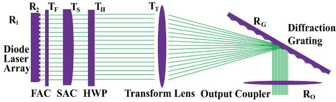
Fig. 1. Schematic diagram of the SBC of a diode laser array.
