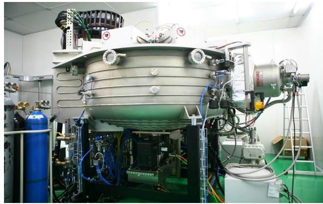
Fig. 11 DC magnetron sputtering system “Nessy 1900.”
