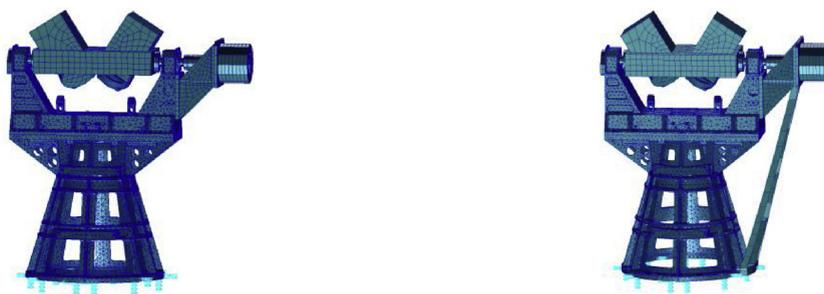
a) without the motor-auxiliary-support      b) with the motor-auxiliary-support
