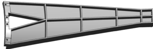
Fig. 6. Final form of the motor-auxiliary-support.
