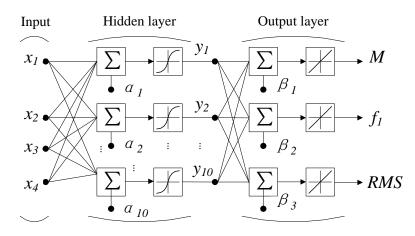
Figure 3 Structure of neural network with one hidden layers and four inputs
