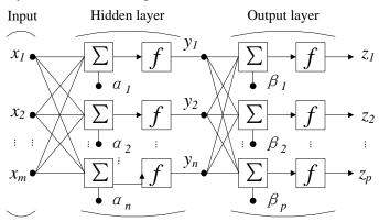
Figure 2 Structure of multi-layer neural network with one hidden layer The process of input signal forward-propagation is as follows,
