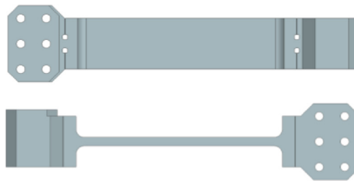
Fig. 5. Model of the tangential constraint structure.
