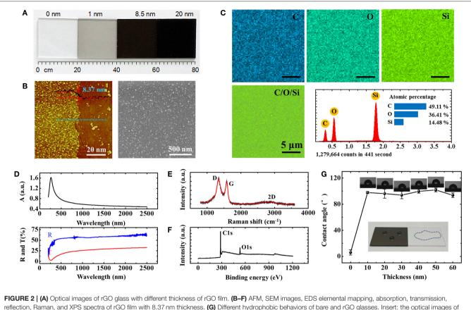
reflection, Raman, and XPS spectra of rGO film with 8.37 nm thickness. (G) Different hydrophobic behaviors of bare and rGO glasses. Insert: the optical images of hydro-phobic and -philic properties of the 8.37 nm rGO and bare glass, respectively.
