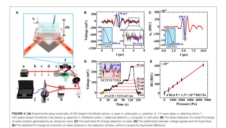
reflection difference between TM and TE modes caused by the variation of RI in microfluidic environment can be captured and recorded in an accurate way. Therefore, in our experiment, when the pressure of liquid (water,  $n_2 = 1.33$ ) in microfluidic channel changes, the RI of the medium will be varied accordingly, and it can also be measured by the photo detector (Xing et al., 2014; Wang et al., 2018).
