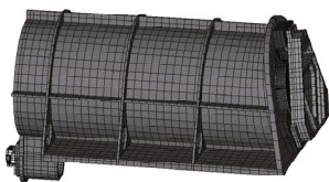
(a) Structure of the laser communication terminal
