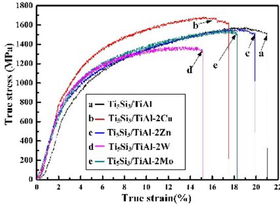
Fig. 3. (Color online) Compression true stress–strain curves.
