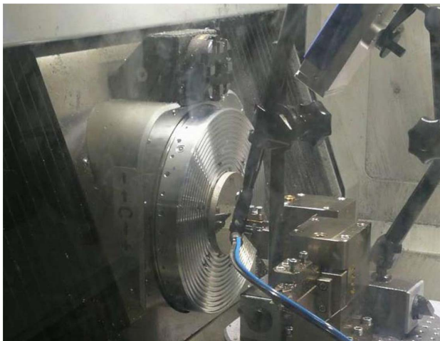
Fig. 1. Process of NiP layer by SPDT.
