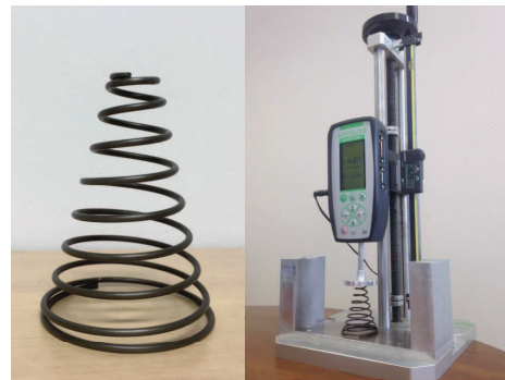
Fig. 12. Conical spring manufactured and measuring equipment
