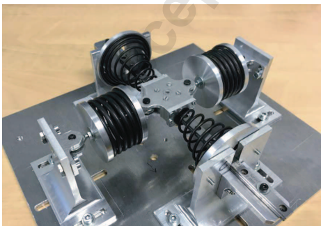
Fig. 14. NES system with linear springs of large mean diameter
