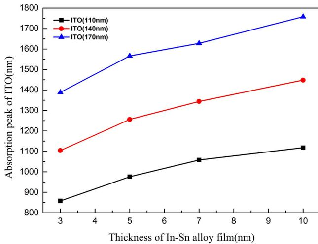
**Figure 5.** The LSPR wavelength shift of ITO NPs as a function of the In-Sn alloy film.
