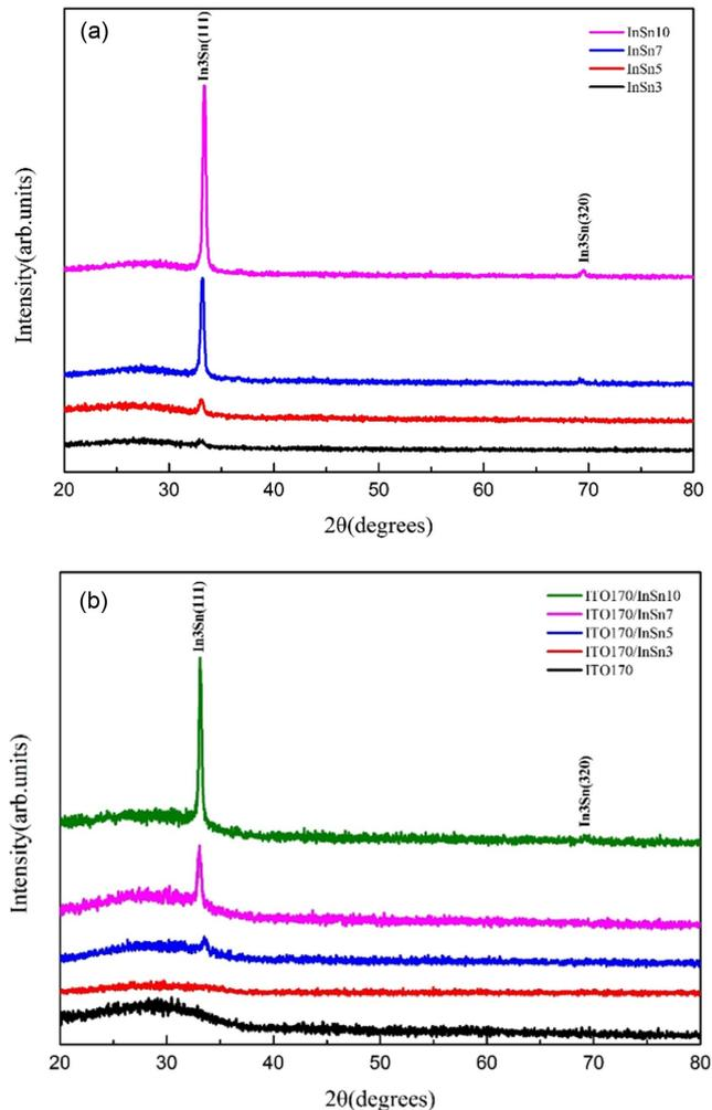
**Figure 2.** The representative XRD patterns of (a) the single In-Sn layer and (b) the ITO/In-Sn bilayer films.
