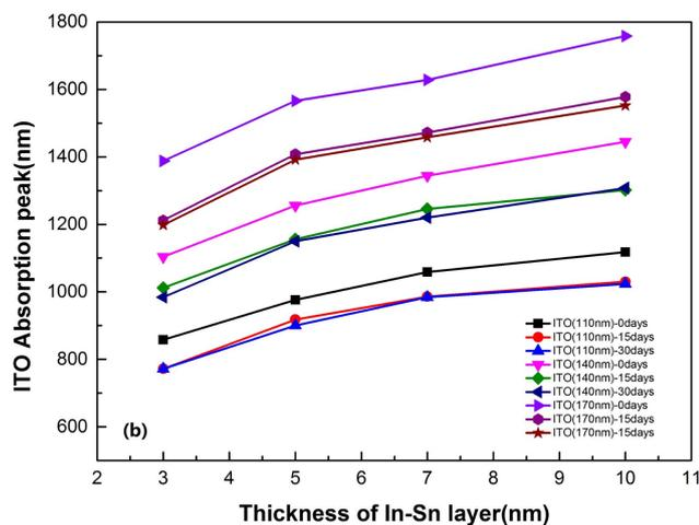
**Figure 6.** The LSPR wavelength shift of ITO NPs in air exposure for 15 d and 30 d: (a) a representative sample of ITO(110 nm)/In-Sn(3 nm) for LSPR shift; (b) the LSPR shift for all samples after air exposure.
