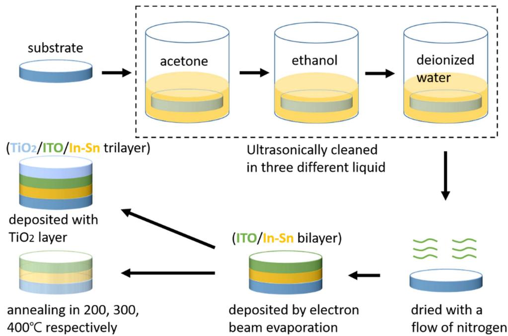
Figure 1. A schematic diagram of the whole experiment.
