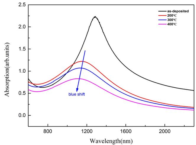
**Figure 7.** A representative sample of ITO(140 nm)/In-Sn(5 nm) for the LSPR shift of ITO NPs after vacuum annealing.
