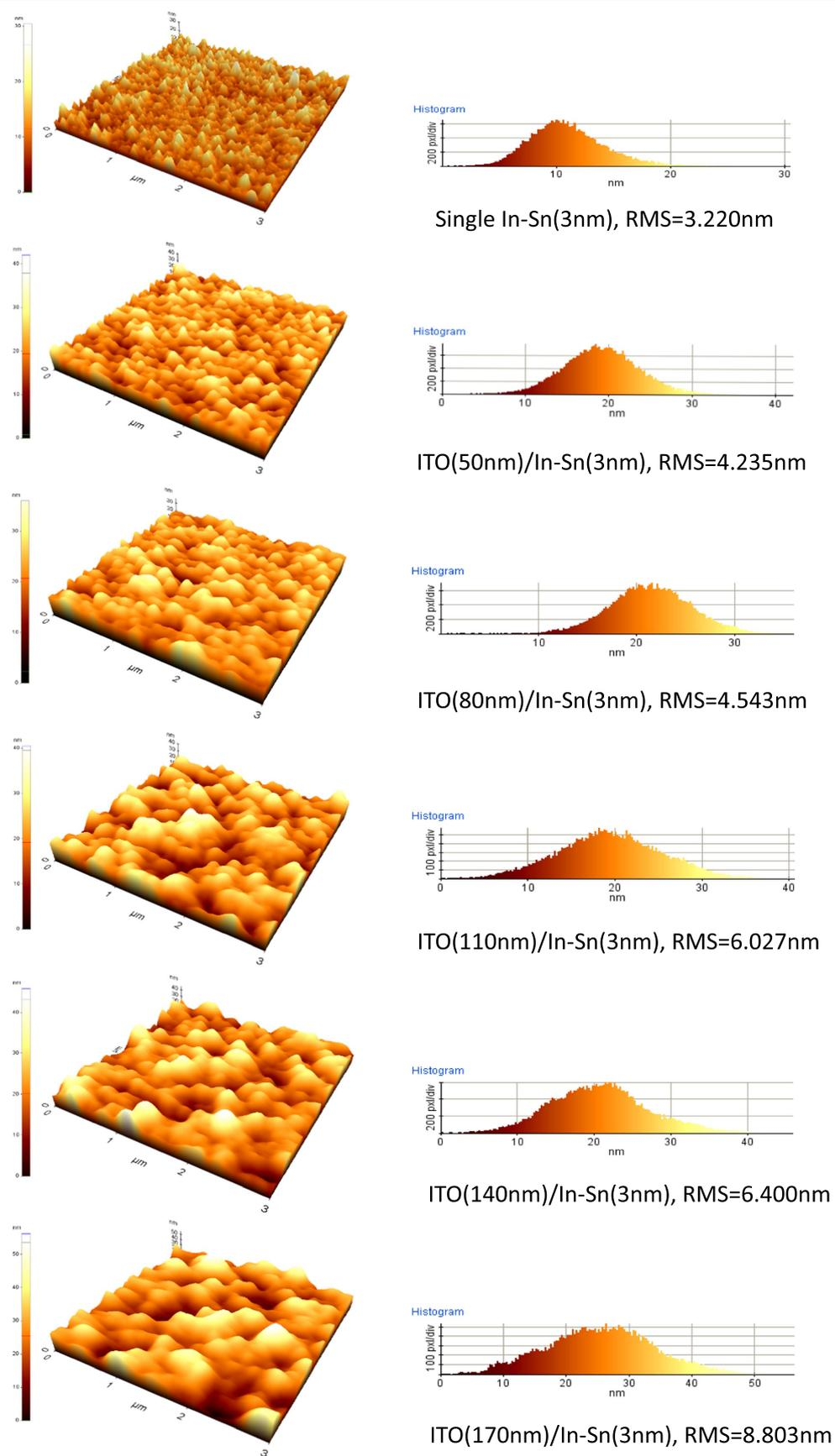
**Figure 3.** Representative AFM images and their corresponding grain height distributions (right column) of ITO/In-Sn NPs as a function of ITO thickness.
