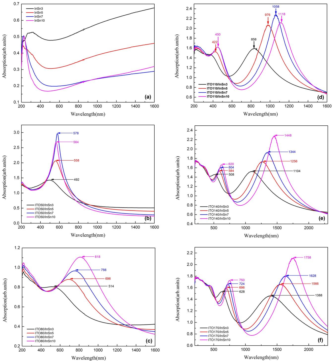
**Figure 4.** The LSPR of ITO in an ITO/In-Sn bilayer structure. Each group has four samples; the thickness of the In-Sn layer was always 3, 5, 7 and 10 nm for a fixed ITO thickness.
