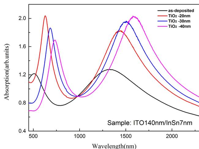
**Figure 8.** A representative sample of ITO(140 nm)/In-Sn(7 nm) for the LSPR wavelength of ITO NPs as a function of the thickness of the  $\text{TiO}_2$  layer.
