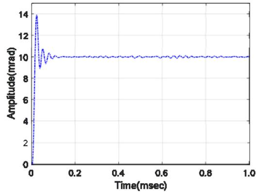
Fig. 5. Step response curve of FSM with PID controller.
