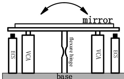
Fig. 1. Structure of a FSM.
