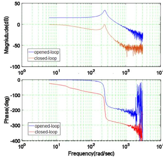
Fig. 2. Frequency responses of the FSM system.
