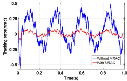
Fig. 11. Angle tracking performance and tracking error.
