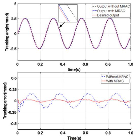
Fig. 10. Angle tracking performance and tracking error.
