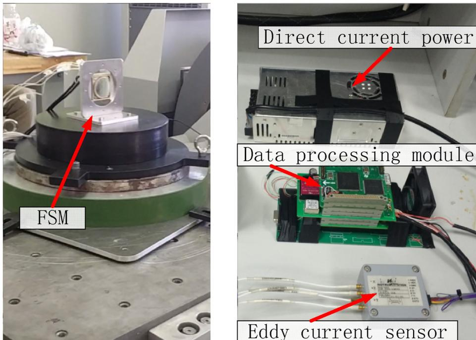
Fig. 8. Photo of the experimental setup.
