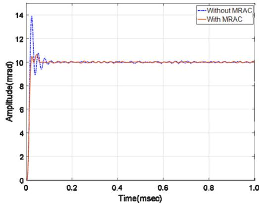
Fig. 9. Closed-loop step response of the FSM.
