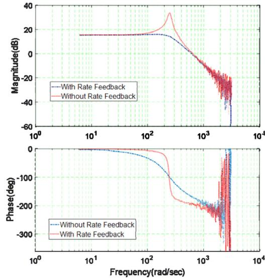
Fig. 4. Open loop frequency responses of the FSM with and without rate feedback.
