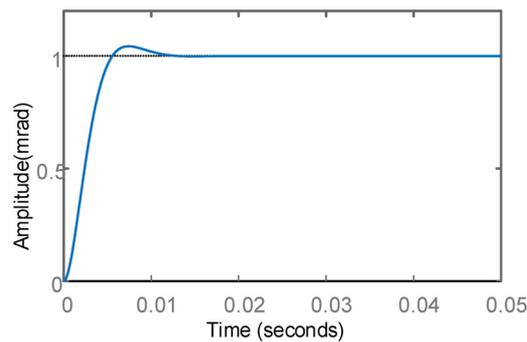
Fig. 6. Step response curve of the reference model.
