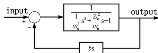
Fig. 3. Block diagram of a second order system with rate feedback.
