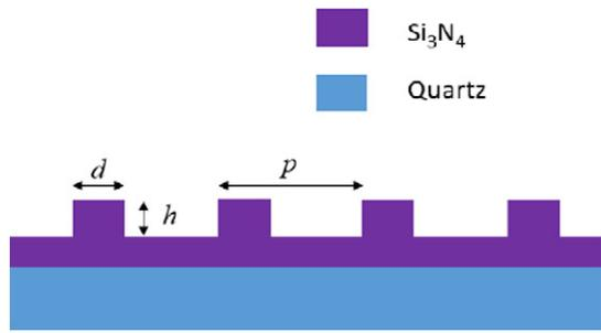
**Fig. 1.** Schematic showing mask design parameters of the silicon nitride gratings for simulation.
