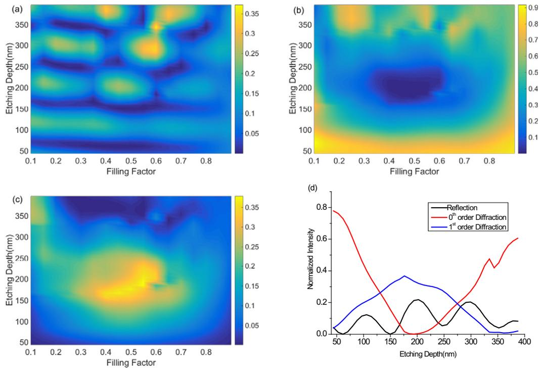
Fig. 3. Simulation results of intensity for back reflection (a), 0th (b) and 1st order diffraction (c) of IPISM-II (period 888 nm). (d) demonstrates the intensities at  $d/p = 0.5$ .
