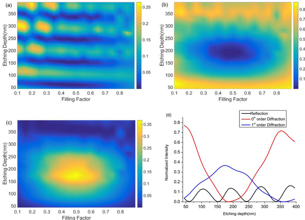
**Fig. 2.** Simulation results of intensity for back reflection (a), 0th (b) and 1st order diffraction (c) of IPISM-I (period 1.776  $\mu\text{m}$ ). (d) demonstrates the intensities at  $d/p = 0.5$ .
