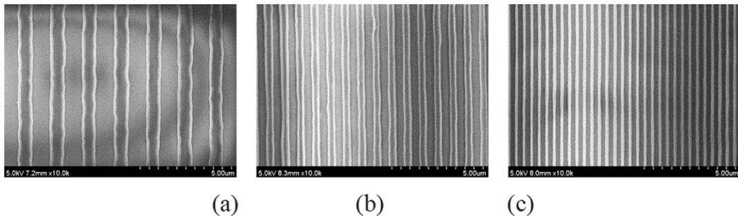
Fig. 4. The SEM pictures of IPISM-I (a), IPISM-II (b), and the target sample (c).
