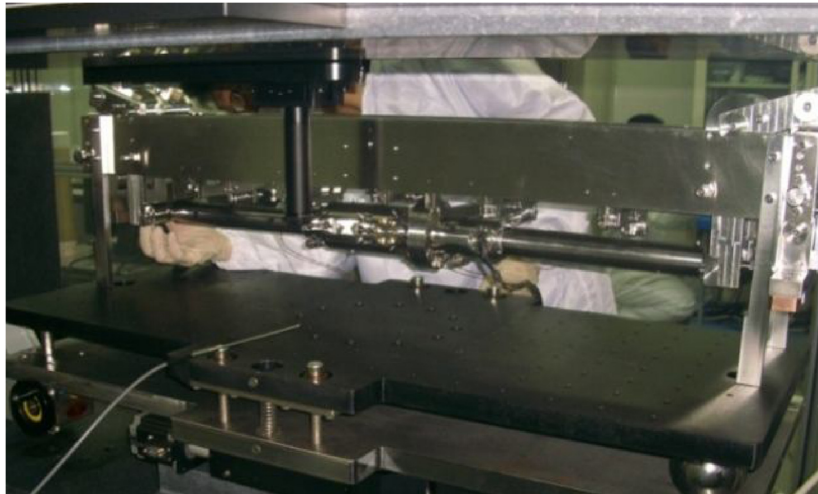
Fig. 21. Photograph showing the surface bending mechanism on the LTP-1200.
