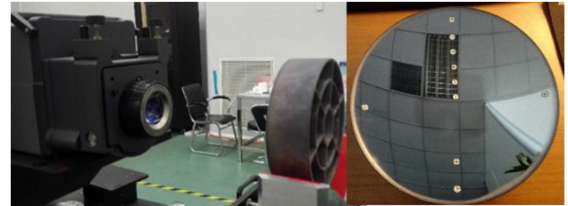
Fig. 6. Distortion calibration of the F0.75 transmission sphere.
