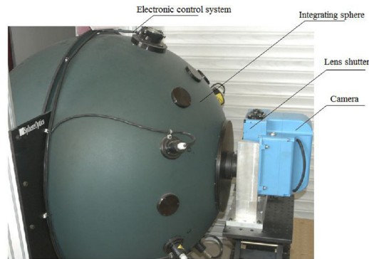
Fig. 9. The measurement of illuminance on the image surface of camera.
