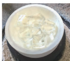
(a) 玻璃塌陷 (a) Collapsed glass
