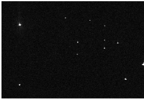
Fig. 3. The actual spectrum of mercury lamp acquired by echelle cross-prism spectrometer.
