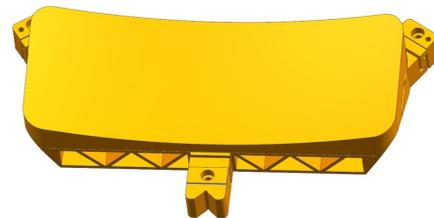
FIG. 3. CAD model of the tertiary mirror.
