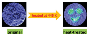
Fig. 6 Photographs of the “smiling face” pattern before and after heat treatment, demonstrating the potential application in the anti-fake field.
