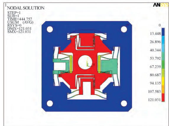
图 9 微位移平台的二阶模态 Fig. 9 Diagram of second-order modal shape of micro-motion stage
