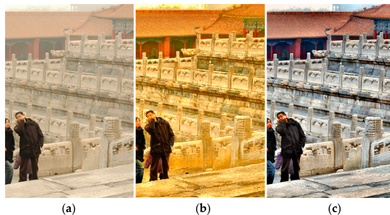
Figure 7. Color casts: (a) the original image needs white balance; (b) the result without white balance; (c) the result with white balance.
