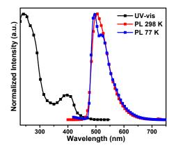
Fig. S2. Normalized UV-vis absorption and emission spectra of  $Ir(BTBP)_2POP$  in degassed  $CH_2Cl_2$  solutions (5 × 10<sup>-5</sup> mol·L<sup>-1</sup>) at room temperature and 77 K.
