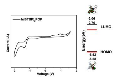
Fig. S4. Cyclic voltammogram curve (left) and contour plots of HOMO/LUMO with theoretical (black) and experimental (red) energy levels (right) of Ir(BTBP)<sub>2</sub>POP.
