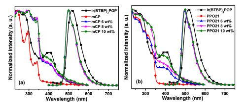
**Fig. S3.** Normalized UV-vis absorption and emission spectra of **Ir(BTBP)<sub>2</sub>POP** in films of mCP (a) and PPO21 (b) with different doping concentration.
