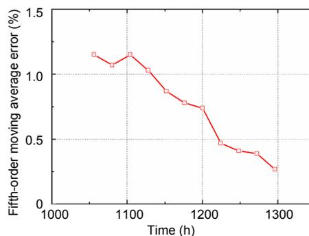
**Fig. 4 Variation of the moving average error versus cut-off time for the test at 80 °C**
