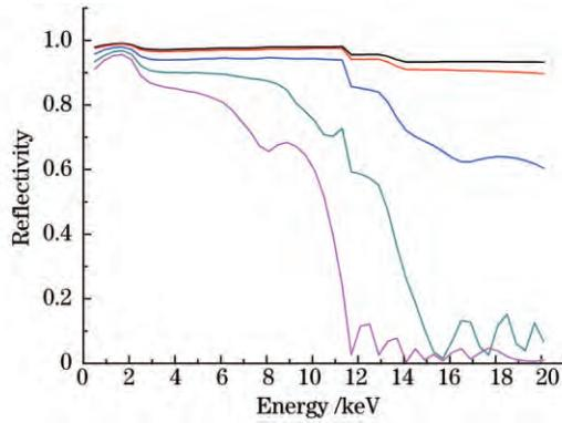
图3 W/B<sub>4</sub>C多层膜不同掠入射角的反射率曲线。曲线由上到下掠入射角依次为:2,5,8,11,14 mradFig.3 Reflectivity curves of W/B<sub>4</sub>C multilayers at different grazing incident angles. The grazing incident angles of the curves from top to bottom is 2,5,8,11,14 mrad, respectively
