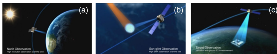
Fig. 2 HRHS-GS observation modes. (a) Nadir mode. In nadir mode, the attitude control system (ACS) points the instrument aperture to the local nadir, so that data can be collected along the ground track just below the spacecraft. (b) Glint mode. In glint mode, the ACS is programmed to point the instrument aperture between the local nadir the bright “glint” spot, where sunlight is specularly reflected from the Earth’s surface. (c) Target mode. In target mode, the ACS points the instrument aperture at specific stationary surface targets as the satellite flies overhead.
