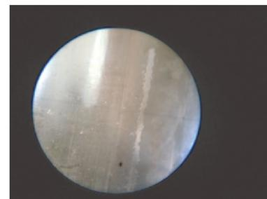
(a) Surface of inner ring before testing
