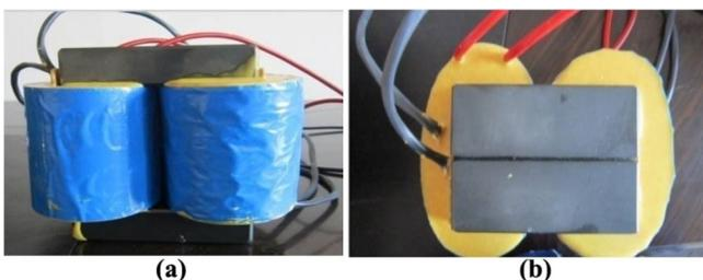
FIG. 5. Prototype of high-voltage pulse transformer.
