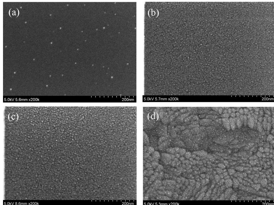
**Fig. 3.** SEM images of (a) 0.5, (b) 0.75, (c) 1 nm Au layers on Si wafers, and (d) 0.75 nm Au layer on an ITO glass substrate.
