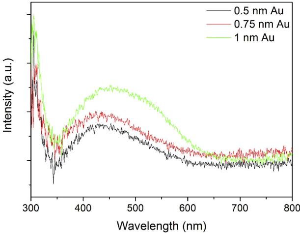
**Fig. 4.** Absorption spectra of Au layers with different thickness on ITO glass substrates.
