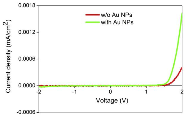
**Fig. 6.** J-V curves of the hole-only devices ITO/MoO<sub>3</sub>/DBP/TAPC/Al with or without 0.75 nm Au.
