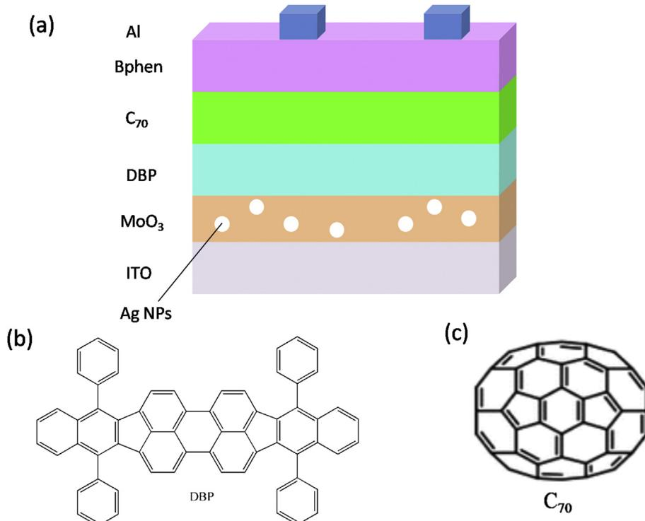
**Fig. 1.** (a) Device structure of the plasmonic OSCs, and the molecular chemical structures of (b) DBP and (c) C<sub>70</sub>.
