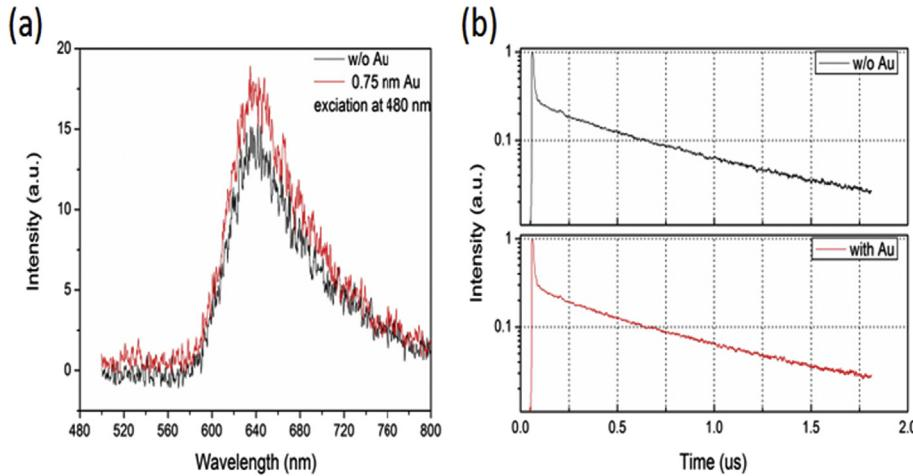
**Fig. 7.** (a) Steady-state PL spectra and (b) transient PL spectra of the MoO<sub>3</sub>/DBP films with or without Au NPs.
