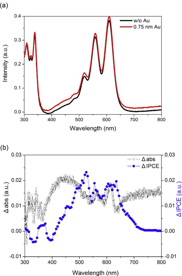
**Fig. 5.** (a) Absorption spectra of the ITO/(Au)/MoO<sub>3</sub>(the optimized thickness)/DBP(60 nm) films without and with 0.75 nm Au layer, (b)  $\Delta\text{abs}$  of the films and  $\Delta\text{IPCE}$  of the devices with and without Au NPs.
