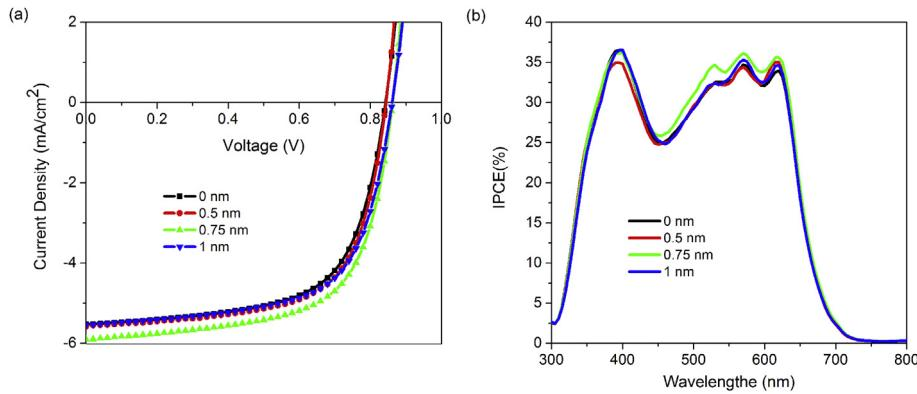
**Fig. 2.** (a) J-V curves and (b) IPCE spectra of the optimized devices with different thickness of Au layers.
