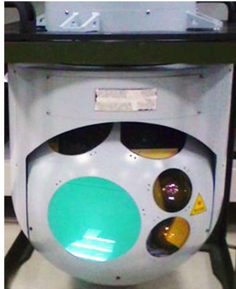
**Fig. 5** Two axes four-gimbal ISP in actual experiments
