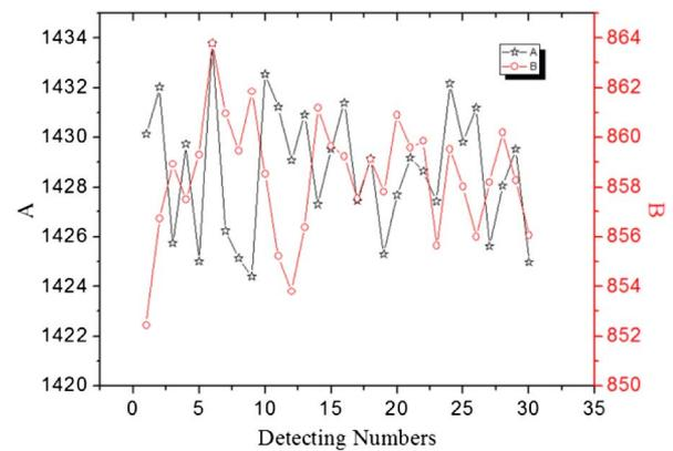
**Fig. 6.** (a) Measured intensity of the peak at 546 nm in the decoded Hg lamp spectrum that used the signal-processing algorithm to remove the crosstalk. (b) Measured intensity of the peak at 546 nm in the decoded Hg lamp spectrum that used the opaque rows.
