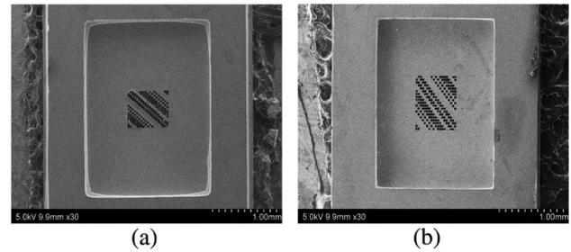
Fig. 4. (a) Coded apertures without opaque rows. (b) The coded apertures with opaque rows.
