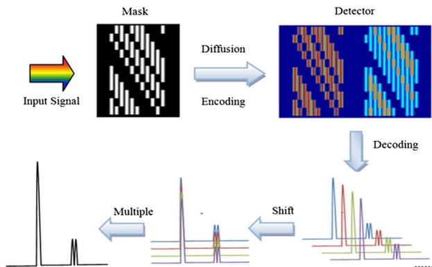
Fig. 1. Encoding and decoding principle of the coded aperture spectrometer.
