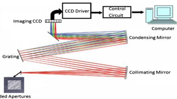
Fig. 3. Schematic of the coded aperture spectrometer.
