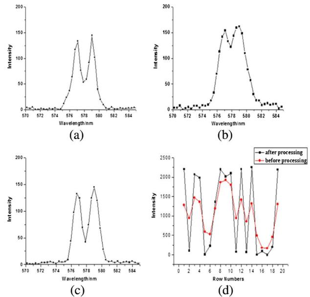
Fig. 5. (a) Decoded spectrum of the Hg lamp using the opaque rows to remove the crosstalk. (b) The spectrum decoded directly from the data without any processing when using the coded apertures without the opaque rows. (c) The decoded spectrum using the algorithm based on deconvolution to remove the crosstalk. (d) The encoded data of one column of pixels before and after removing the crosstalk when using the coded apertures without opaque rows.
