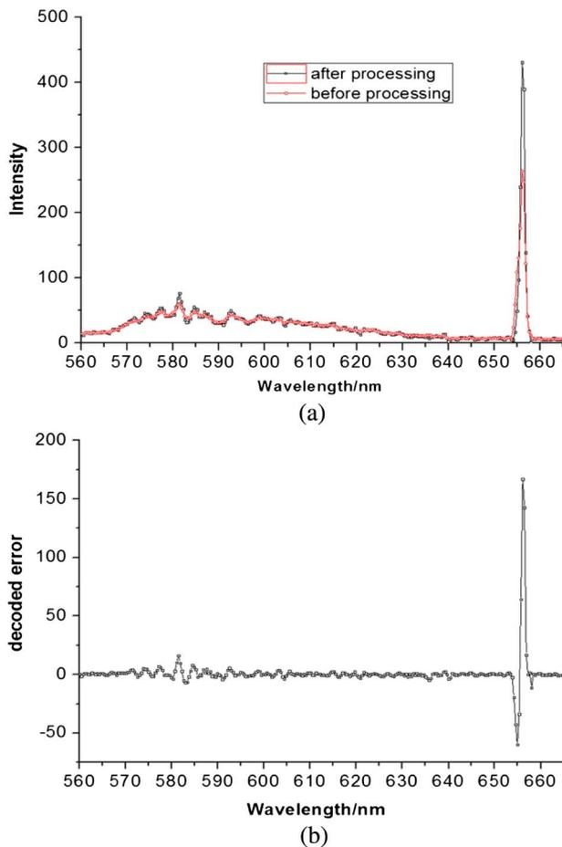
**Fig. 7.** (a) Decoded spectra of the deuterium lamp before and after removing the effect of the crosstalk with the algorithm we proposed. (b) The difference between the two decoded spectra.
