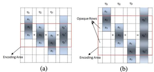
Fig. 2. (a) Schematic of the crosstalk caused by the PSF of the optical system. (b) The schematic of the signal distribution when the opaque rows are placed between the coded apertures.
