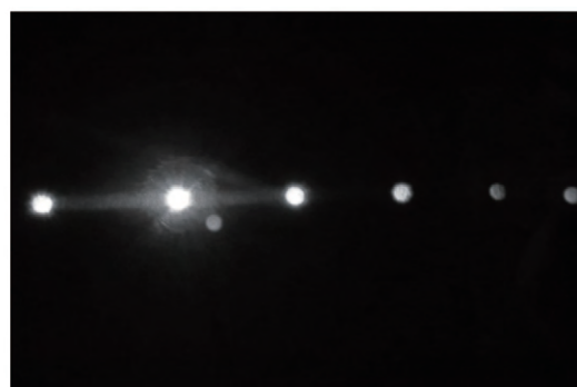
图 9 试刻中阶梯光栅的衍射光斑 Fig.9 Diffraction spots of the echelle grating in the experiment
