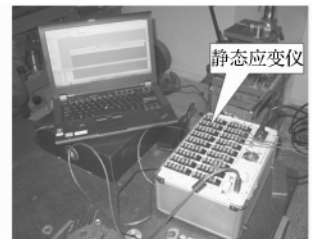
图 7 DH3815 静态应变仪 Fig. 7 DH3815 static strain instrument
