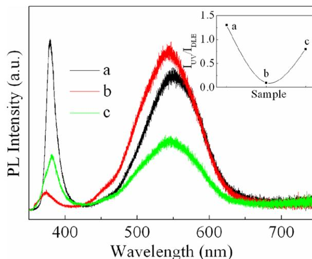
Fig. 4 Room temperature PL spectra of ZnO thin films prepared in different solvents. (a) water, (b) ethanol, and (c) propanol. Inset is the  $I_{UV}/I_{DLE}$  ratio.
