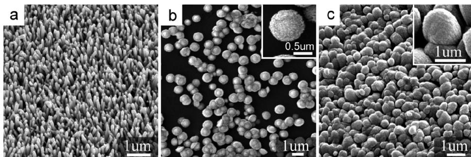
Fig. 2 SEM images of ZnO thin films prepared in different solvents. (a) water, (b) ethanol, and (c) propanol. Insets in (b) and (c) are the enlarged figure of individual crystal, respectively.
