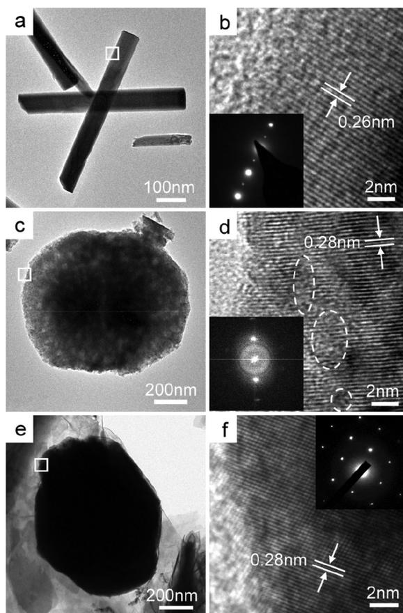
Fig. 3 TEM (left) and HRTEM (right) images of ZnO thin films prepared in different solvents. (a, b) water, (c, d) ethanol, (e, f) propanol. Insets are the corresponding SAED pattern. The white circles point to the defects.
