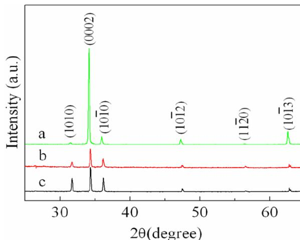
Fig. 1 XRD patterns of ZnO thin films prepared in different solvents. (a) water, (b) ethanol, and (c) propanol.
