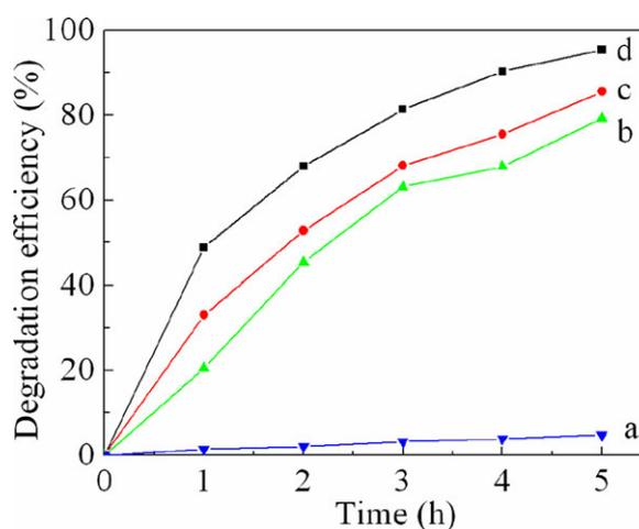
Fig. 5 Photodegradation of RhB under different conditions: (a) without catalyst, (b) microellipses, (c) microdisks, (d) nanorods.
