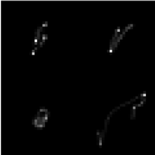
**Fig. 8** Blur kernels.<sup>21</sup> From left to right, top to bottom: PSF1, PSF2, PSF3, and PSF4.
