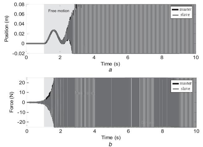
**Fig. 5** Results when the SMADOs work as robust compensators
