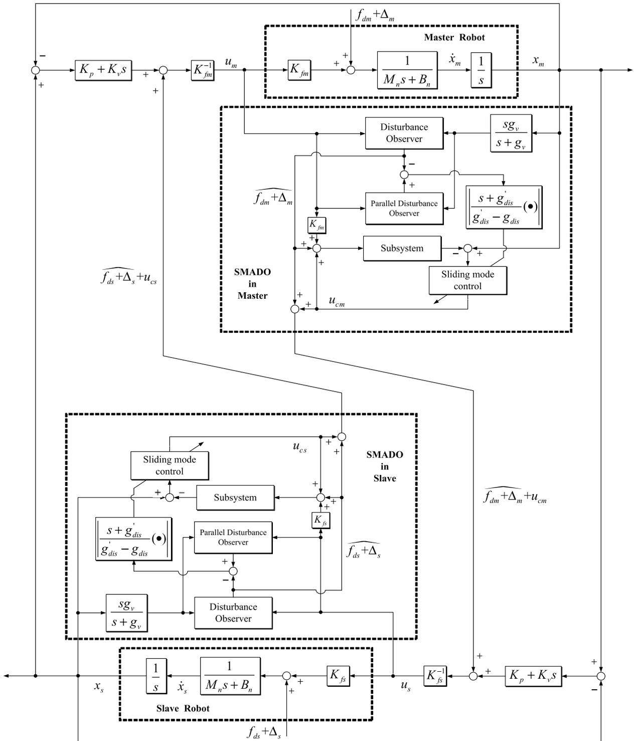
Fig. 3 DOB-based four-channel bilateral control structure
