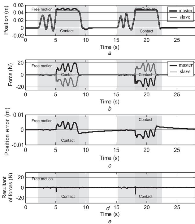
**Fig. 8** Results of sensing the rigid object by conventional DOB
