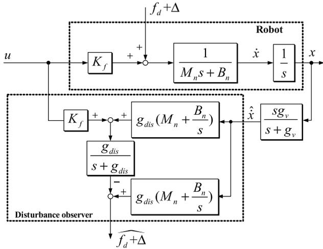
Fig. 2 Block diagram of DOB
