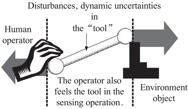
**Fig. 1** Haptic sensing system with tolerated disturbances and uncertainties
