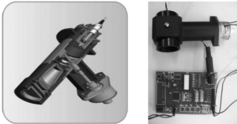
Fig. 3. Coarse/fine beacon switching equipment.
