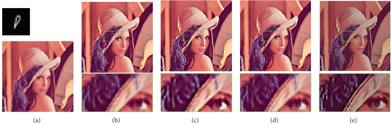
FIGURE 7: Superresolution reconstruction for the Lena image. (a) The input “Lena” image degraded by kernel-1. The result of reconstructed HR image by using (b) DCCI method [6], (c) FIU method [22], and (d) ScSR method [10], respectively, from the deblurred LR image with the AMAP algorithm [23]. (e) The result of our method directly from the blurred LR image.
