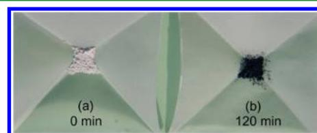
Figure 3.  $\text{TiO}_2$  powder before and after laser modification. (a) Raw  $\text{TiO}_2$  and (b)  $\text{TiO}_2\text{-}120$ .
